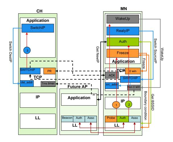
Figure 15. IPMN-Fast Handoff Architecture and event sequencing for overlapping cell boundary condition.
