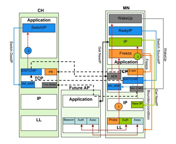
Figure 16. IPMN-Normal Handoff Architecture and event sequencing for non-overlapping cell boundary condition.
