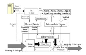
Fig-2 EDIP Selective Decapsulation System
