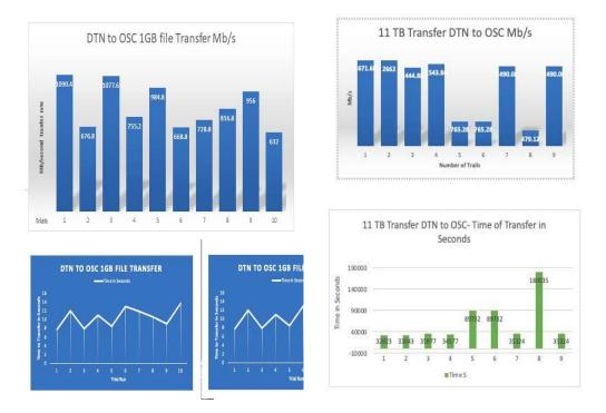
Fig-4 Transfer rate and time for moving 1TB (left diagrams) and 11 TB (right two diagrams) files between DTNs of Kent and OSC
